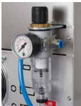
Forced cooling system with compressed air
