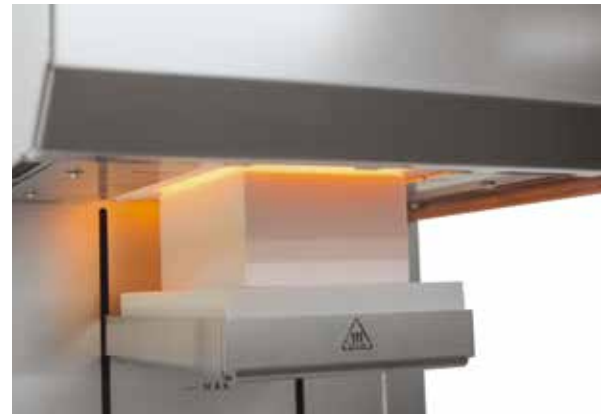
Automated table lowering for cooling
